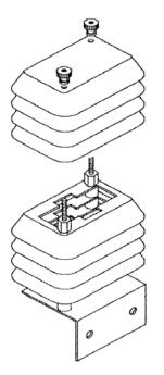
**Important:** External sensor wires connect to the logger from the side at the point where the top and bottom sections meet. Secure the external sensor wires to the mast just below the radiation shield with a plastic tie to ensure that the sensor wires do not become disconnected while recording.
